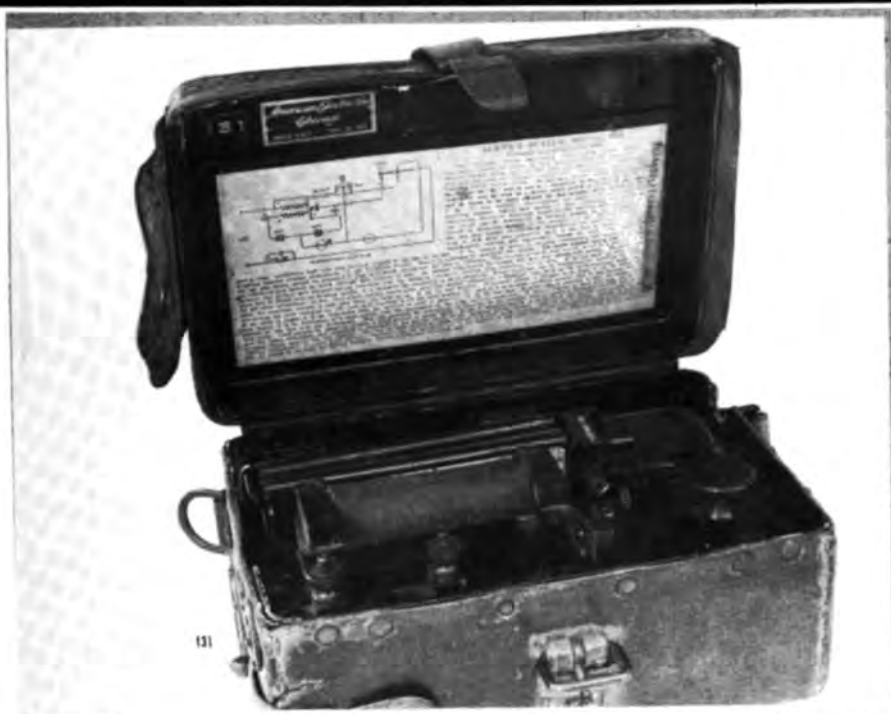
● (131) Service buzzer. U.S. Signal Corps, Model 1914. Mr Mfr. American Electric Co. Chicago.
